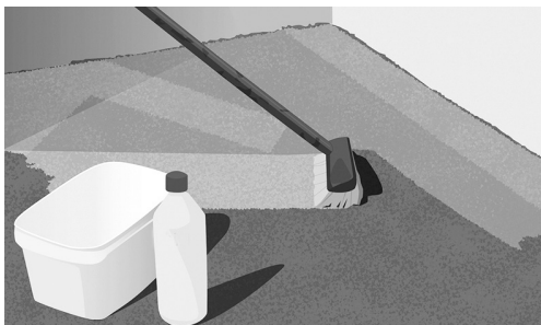
Fig. 7. Clean and pre-treat the floor.
